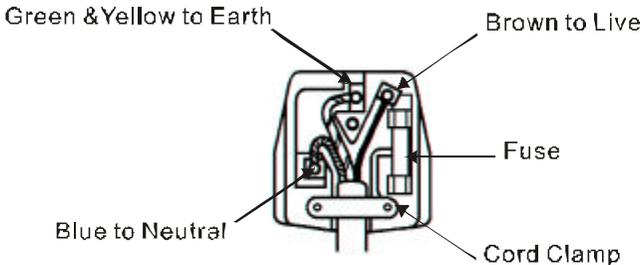
The wire which is coloured GREEN and YELLOW must be connected to the terminal in the plug which is marked with the letter E or by the earth symbol  $\oplus$  or coloured GREEN or GREEN and YELLOW.
